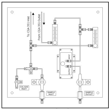
Figure 1-3: Typical Sample System
