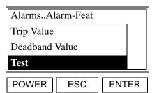
Use the  $[\blacktriangle]$  and  $[\blacktriangledown]$  keys to select [Test], and press [ENTER].
