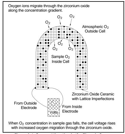
Figure 1-4: Oxygen Migration in the Zirconia Sensor
