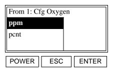
A list of the available unit types is shown. Use the [▲] and [▼] keys to select the desired units (*parts per million* or *percent*) and press [ENTER].
