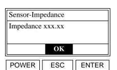
The oxygen sensor impedance, in ohms, is shown. Press [ENTER] to continue.
