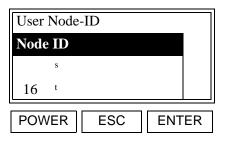
Use the [▲] and [▼] keys to scroll the list of available node ID numbers. When the desired number is highlighted, press [ENTER].
