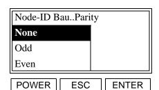
Use the  $[\blacktriangle]$  and  $[\blacktriangledown]$  keys to select the parity setting and press [ENTER].
