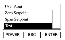
Use the  $[\blacktriangle]$  and  $[\blacktriangledown]$  keys to select [Test], and press [ENTER].
