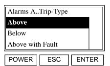
Use the  $[\blacktriangle]$  and  $[\blacktriangledown]$  keys to select the desired trip type, and press [ENTER].
