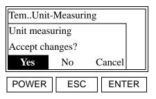
This message indicates that changes in this menu will alter the live data output. To accept the new value, use the [◀] and [▶] keys to select [Yes] and press [ENTER].
