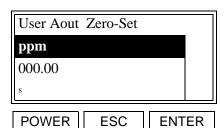
Use [◀] and [▶] to position the cursor under the desired character. Then, use [▲] and [▼] to increment the value. Press [ENTER] when done.
