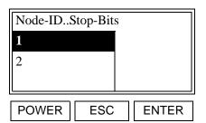
Use the  $[\blacktriangle]$  and  $[\blacktriangledown]$  keys to select desired number of stop bits and press [ENTER].
