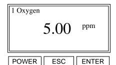
The value shown is now the correct ppm value for the oxygen content of the calibration gas.
