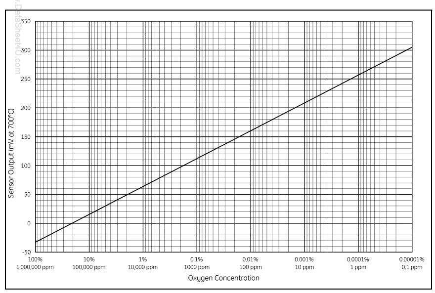
Figure A-1: Oxygen Sensor Output at 700°C
