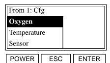
A list of the available display inputs is shown. Use the [▲] and [▼] keys to select the desired input and press [ENTER]. *Oxygen* has been selected as an example.
