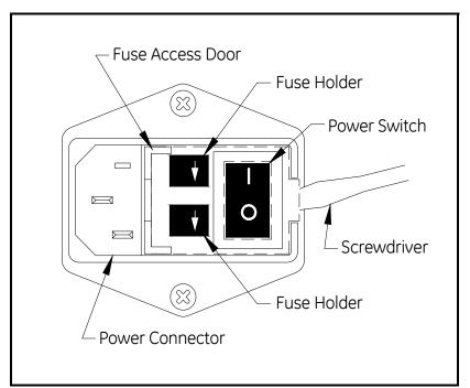
Figure C-4: Rack Mount Fuse Locations
