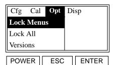
Use the  $[\blacktriangle]$  and  $[\blacktriangledown]$  keys to select the desired option and press [ENTER].
