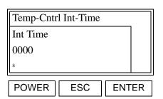
Using the [◀] and [▶] keys, position the cursor under the desired character. Then, use the [▲] and [▼] keys to increment the value. When done, press [ENTER].
