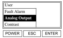
Use the  $[\blacktriangle]$  and  $[\blacktriangledown]$  keys to select [Analog Output] and press [ENTER].
