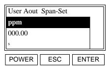
Use  $[\blacktriangleleft]$  and  $[\blacktriangleright]$  to position the cursor under the desired character. Then, use  $[\blacktriangle]$  and  $[\blacktriangledown]$  to increment the value. Press  $[\mathsf{ENTER}]$  when done.
