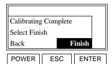
If the calibration passed, use the [◀] and [▶] keys to select [Finish] and press [ENTER].
