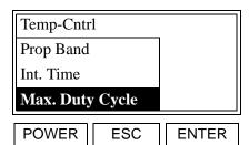
Use the  $[\blacktriangle]$  and  $[\blacktriangledown]$  keys to select [Max. Duty Cycle] and press [ENTER].
