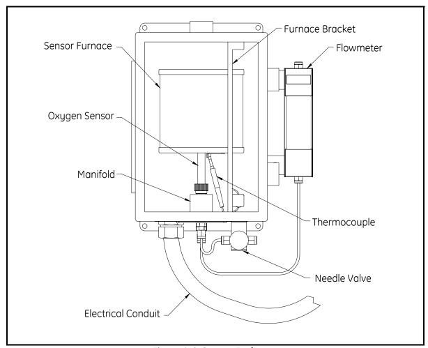
Figure 1-2: Sensor Enclosure
