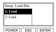
Use the  $[\blacktriangle]$  and  $[\blacktriangledown]$  keys to select the desired slot designation and press [ENTER].
