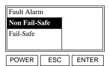
Use the  $[\blacktriangle]$  and  $[\blacktriangledown]$  keys to select the desired alarm type and press [ENTER].
