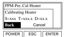
This message appears until the calibration adjustment has been completed (usually about 15–30 minutes).
