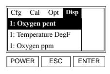
A list of the available windows is shown. Use the  $[\blacktriangle]$  and  $[\blacktriangledown]$  keys to select the desired window and press [ENTER].
