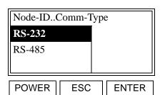
Use the  $[\blacktriangle]$  and  $[\blacktriangledown]$  keys to select type of serial port and press [ENTER].
