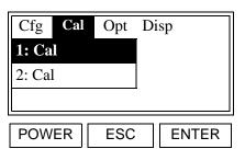
A list of the slots available for calibration is shown. Use the [▲] and [▼] keys to select [1: Cal] and press [ENTER].
