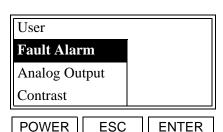
Use the  $[\blacktriangle]$  and  $[\blacktriangledown]$  keys to select [Fault Alarm] and press [ENTER].
