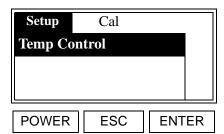
Use the  $[\blacktriangle]$  and  $[\blacktriangledown]$  keys to select [Temp Control] and press [ENTER].
