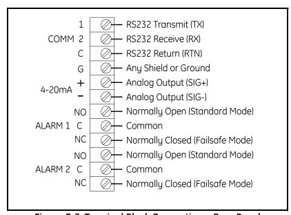
Figure C-3: Terminal Block Connections- Rear Panel
