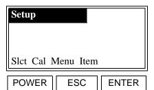
Use the  $[\blacktriangle]$  and  $[\blacktriangledown]$  keys to select [Setup] and press [ENTER].
