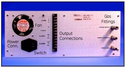
Figure C-2: CGA 351 Rack Mount Version - Rear Panel
