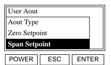
Use the  $[\blacktriangle]$  and  $[\blacktriangledown]$  keys to select [Span Setpoint], and press [ENTER].
