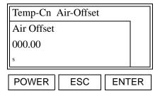
Using the [◀] and [▶] keys, position the cursor under the desired character. Then, use the [▲] and [▼] keys to increment the value. When done, press [ENTER].
