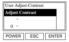
Use the [▲] and [▼] keys to increment the value to a number between 35 (min. contrast) and 50 (max. contrast). When done, press [ENTER].
