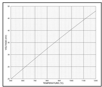
Figure 5-1: TC Voltage vs. Temperature
