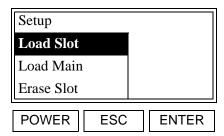
Use the  $[\blacktriangle]$  and  $[\blacktriangledown]$  keys to select the desired action and press [ENTER].
