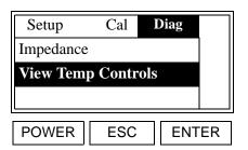
Use the  $[\blacktriangle]$  and  $[\blacktriangledown]$  keys to select [View Temp Controls] and press [ENTER].
